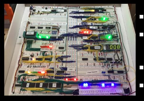
Custom 8-bit computer Based on project by **Ben Eater** Work in progress! 6502, but simpler
