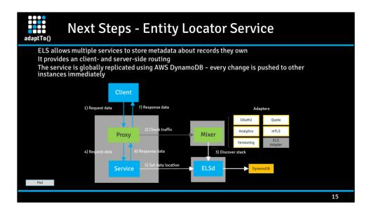
Proxy: Istio uses an extended version of the Envoy proxy, a high-performance proxy developed in C++, to mediate all inbound and outbound traffic for all services in the service mesh.
