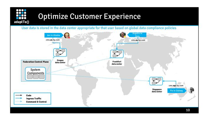
User signs up for an HP application or service, their data gets stored in the data center that is appropriate based on the global data compliance policies that are implemented as part of the service mesh or policy enforcement.
